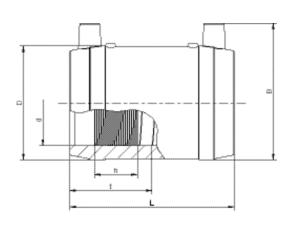
PE 100 SDR 7.4 Maximum working pressure 25 bar (water)
