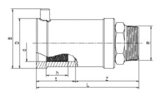
PE 100 SDR 11 Maximum working pressure 16 bar (water)
