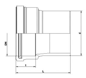
PE 100 Maximum testing pressure 0.5 bar in accordance to DIN EN 1610
