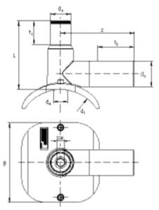
PE 100 SDR 11 Maximum working pressure 16 bar (water)/10 bar (gas)
