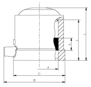
PE 100 SDR 11 Maximum working pressure 16 bar (water)/10 bar (gas)
