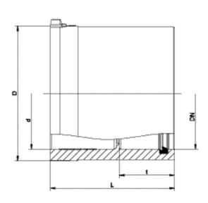
Maximum permissible test pressure 0.5 bar to DIN EN 1610
