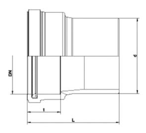
PE 100 Maximum permissible test pressure 0.5 bar to DIN EN 1610
