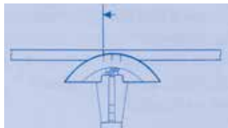
Phase 2 - Place the pipe inside the bending clamp.
